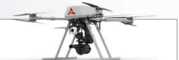
GRENADED WITH 6 GRENADE LAUNCHERS AND GIMBAL CAMERA OPTION
